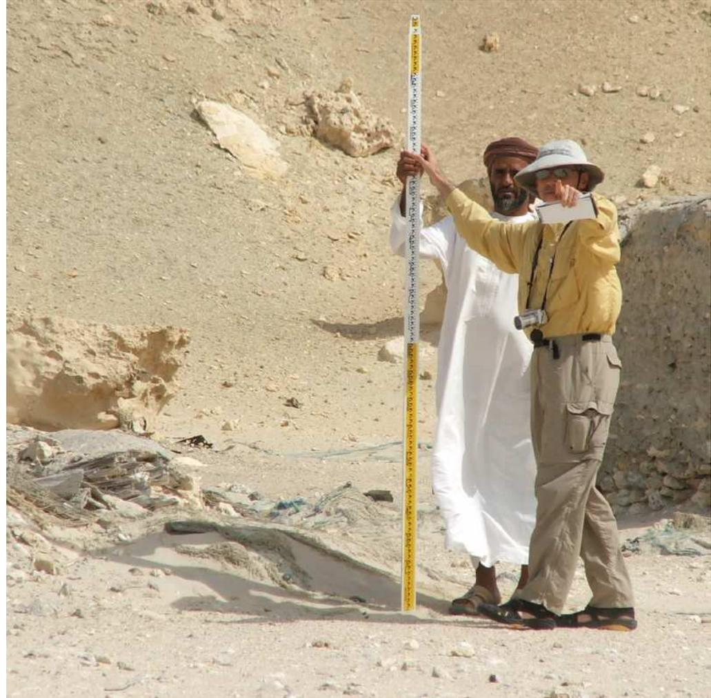
**Figure 2.:** Surveying techniques demonstrated at Ras al Duqm (Site 31). Professor Fritz uses laser ranger at coast line (*left*), while 43 m away, Professor Raad and tsunami witness Mr. Soubayh bin Rajid bin Sa'id Al-Joubaybi identify site of maximum penetration with surveying rod (*right*), defining run-up of 2.6 meters.
