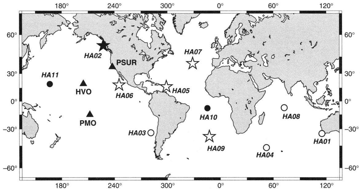
▲ **Figure 1.** Map of the hydroacoustic network of the IMS, including hydrophone stations (circles) and *T*-phase stations (stars). Solid symbols indicate operational sites, open ones are planned. Stations are identified by their IMS codes. The triangles indicate other sites, not part of the IMS, described in the text.
