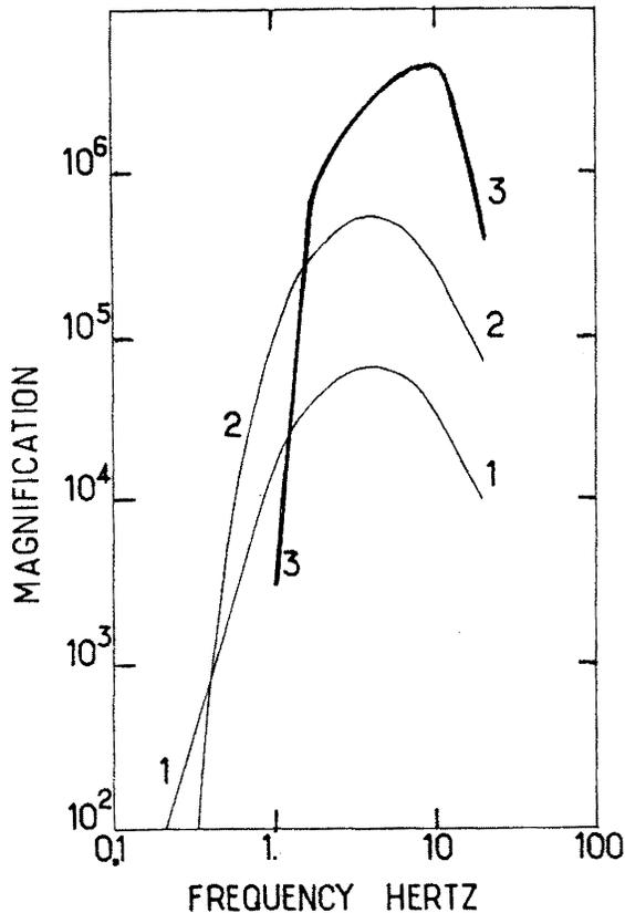
▲ **Figure 4.** Magnification curves for analog channels of the RSP. 1: Standard, low-gain short-period channel; 2: High-gain short-period channel with high-pass filter ( $f \geq 0.3$  Hz) rejecting sea swell; 3 (thick curve): “*T*-wave channel” band-passed between 1 and 10 Hz, with typical magnification of  $2 \times 10^6$  at 3 Hz. After Talandier and Kuster (1976).
