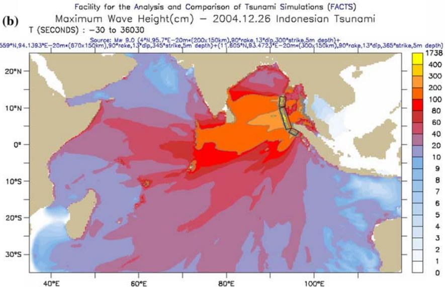
**Fig. 1** (a) Map of the Indian Ocean locating Socotra off the Horn of Africa. Distances from the epicenter of the 2004 Sumatra–Andaman earthquake (red star) are shown for companion surveys: Sri Lanka (Liu et al. 2005), Maldives (Fritz et al. 2006a, b), Oman (Okal et al. 2006a, b, c) and Madagascar (Okal et al. 2006a, b, c). (b) MOST-tsunami model simulation: maximum computed wave heights in cm (Titov et al. 2005)
