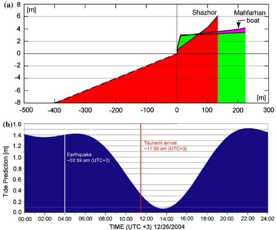
**Fig. 7** (a) Selected cross-shore transects surveyed at Shazhor (maximum runup  $R = 6.1$  m, inundation  $I = 132$  m) and Mahfarhan ( $R = 4.2$  m,  $I = 224$  m), bathymetry estimated from Royal Navy nautical charts (UK); (b) Astronomic tide level prediction for 26 December 2004 at Shiq along Socotra's north shore (4 km northeast of Hadiboh) with time of earthquake off Sumatra and estimated tsunami arrival at Socotra in local time (UTC + 3)
