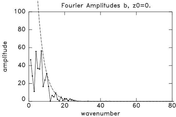
Figure 1: The Fourier spectrum of the vertical component of the magnetic field along the  $180^\circ$  meridian showing the exponential decay with increasing wave number. The dashed curve is the decay that would be expected from surface sources.
