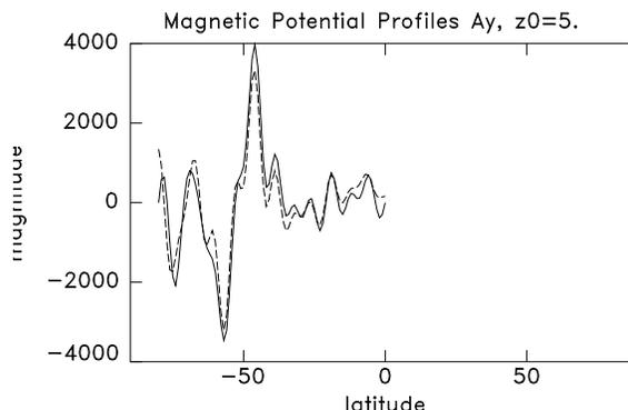
Figure 4: The magnetic potentials generated by integrating the horizontal (dashed) and vertical (solid) magnetic fields along latitude. They are nearly identical, i.e. the magnetic field is nearly two-dimensional in this region.
