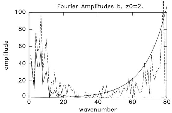
Figure 2: The Fourier spectrum of the vertical component of the magnetic field extrapolated downward about 120 km. The amplification of the noise components and the minimum in the spectrum near wavenumbers  $k=25-30$  are evident. The smooth curve is a fit to white noise extrapolated downward.
