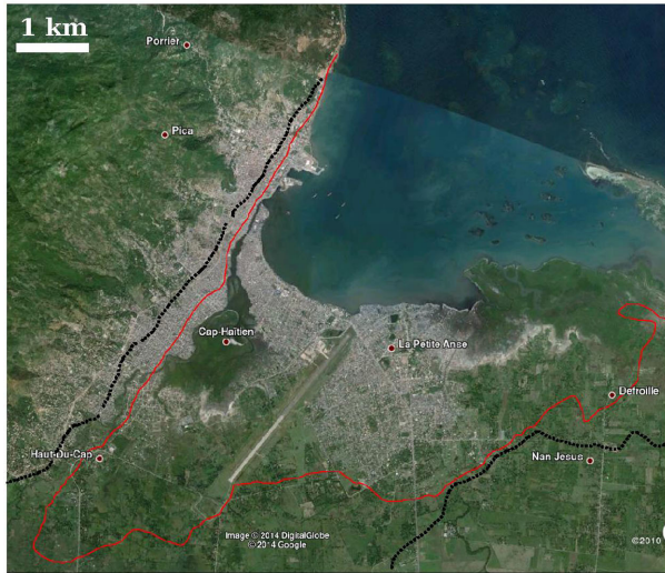
Figure 7. Maximum flooding extent resulting from our calculation reported on the GoogleEarth image of Cap Haitien [left] and of the Caracol development zone [right] (data SIO, NOAA, US Navy, NGA, GEBCO. Image © 2015 DigitalGlobe © 2015 Google). Solid red line: inundation limit for scenario 2; dashed black line: inundation limit for scenario 3.
