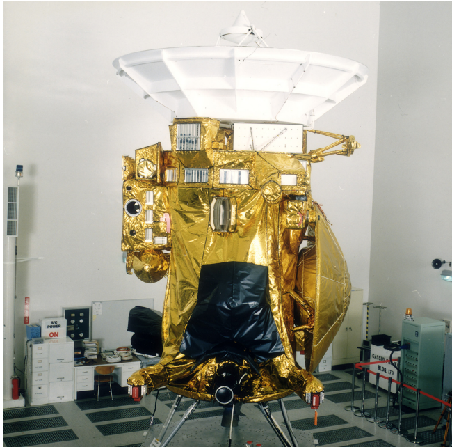
Figure 2.6. The Cassini spacecraft is the largest interplanetary probe to date, measuring 6.8 m in length. The large cone-shaped object on the right is the protective atmospheric aeroshell for the European-managed Huygens probe. The 4 m dish antenna is both a communications device and a scientific instrument in its own right. Some of the optical cameras are visible at left. Image Credit: NASA/JPL.
