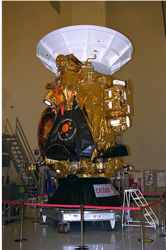
Figure 1.1. The Cassini spacecraft, nearly in flight configuration. The radioactive isotope thermoelectric generators (RTGs) have not yet been installed. The gold wrapping is thermal insulation to help the spacecraft regulate the temperature of its computers and instruments. Image Credit: NASA/JPL.
