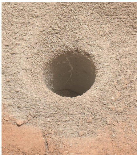
Image taken by the Mars Hand Lens Imager of the John Klein drill hole (1.6 cm in diameter) at Yellowknife Bay reveals gray cuttings of mudstone (ancient lake sediments), rock powder, and interior wall. An array of eight ChemCam laser shot points can be seen. The gray color suggests that reduced, rather than oxidized, chemical compounds and minerals dominated the pore fluid chemistry of the ancient sediment. A cross-cutting network of sulfate-filled fractures indicates later flow of groundwater through fractures after the sediment was lithified.
