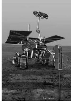
Figure 8.8 ESA's ExoMars mission will consist of a rover and a fixed surface station. The rover, shown in this artist's conception, will be able to drill to depths of 2 m to determine if life might exist underground. (ESA/AOES Medialab.)
